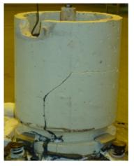
Fig.18. Crucible crack during the test.
