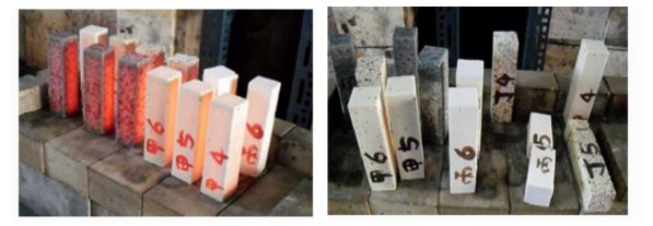
Fig.15. The thermal shock damage test for crucible refractories (left: heated, right: cold).
